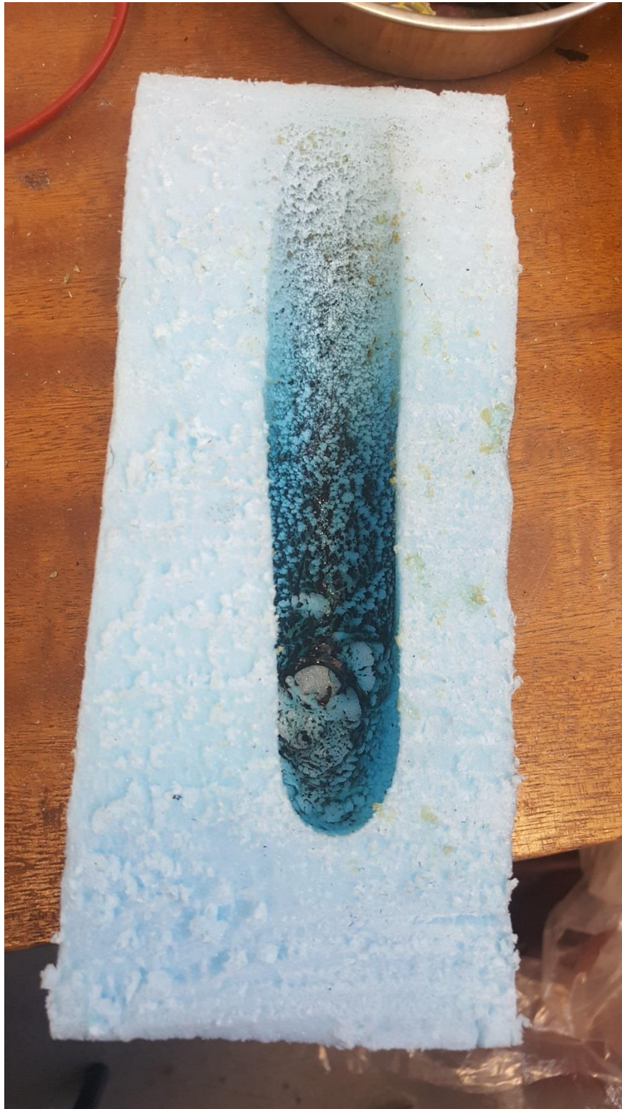
Photograph 8: Sample of the insulating foam from the Medina House cladding panels subjected to single-flame source surface ignition test.
