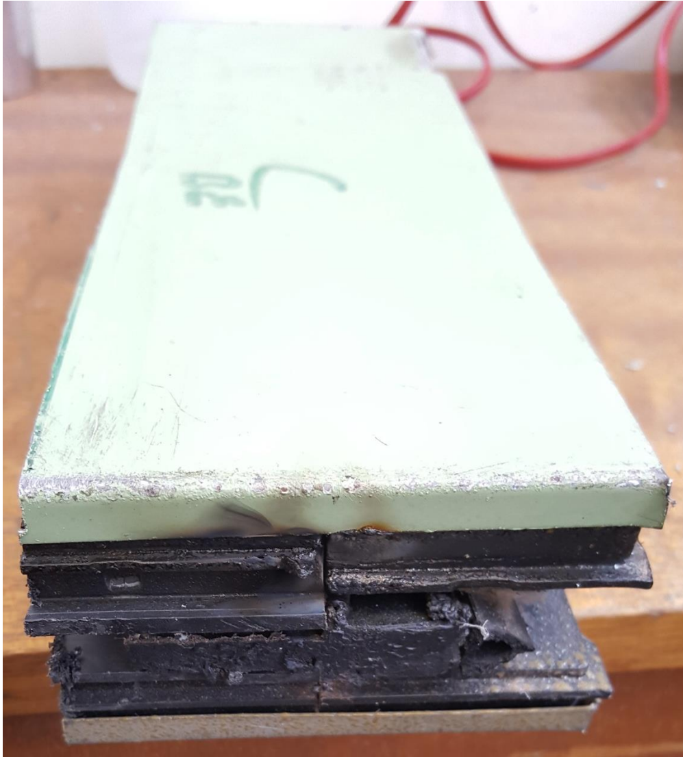
Photograph 7: Sample from Medina House cladding following single-flame source bottom edge ignition test.
