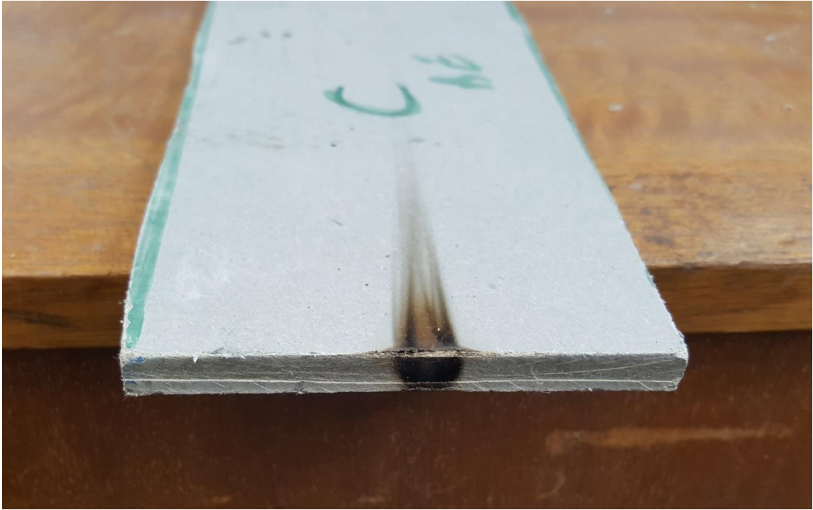
Photograph 5: Sample from Canute Garden cladding following single-flame source bottom edge ignition test.
